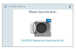
After the door has been closed, the display returns to the default view. The door is locked pressure-tight upon program start.
