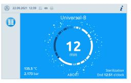
During the program run, the display shows the current program duration, the current parameters and the expected end of the program.
