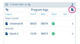
2. Press the button with the arrow to view and output a log.
