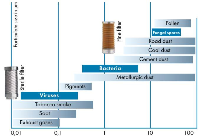
Although Dürr Dental sterile filters do not produce sterile air, they come with a 0.01 µm filter mesh size.
