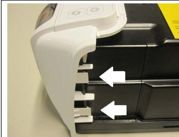
Press the two tabs on the right and left side to release the cover and remove it.
