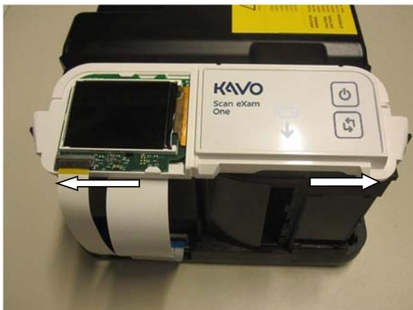
Pull both right and left side locking clips and lift the control panel assembly up
