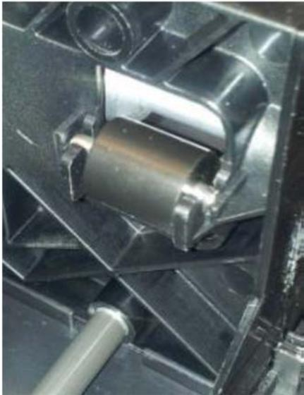
Add the dowel pin to the small wheel and install it to its place.
