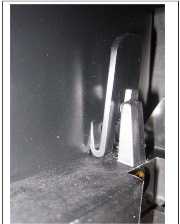
There should not be space between the light cover and chassis. The clip spring force locks the clip hole to the
