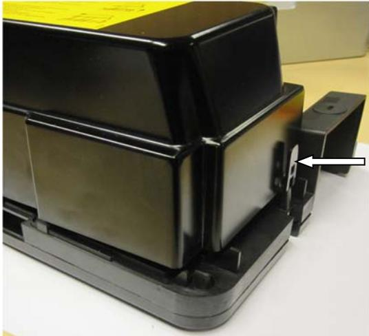
Press the tab on back side and lift the cover up and backwards to remove the light cover
