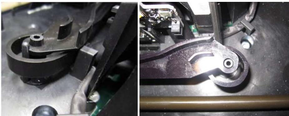
8. Check door operation by rotating the big wheel. When carriage moves forward it should open the door and when backwards the door should be closed.
