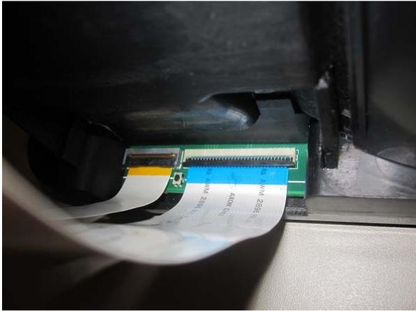
First lift the both connector locking tabs up, then pull the cables out from the connector.
