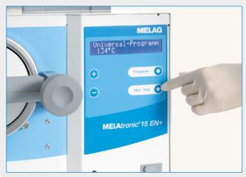
The MELA*tronic*®15 EN+ provides four sterilization programs. The Quick-Program (134 °C) is suitable for unwrapped instruments and takes only 10 minutes (drying extra). The Universal-Program (134 °C) and the Prion-Program (134 °C) also provide quick turnaround times. The Gentle-Program works at lower temperatures (121 °C) and is especially suitable for thermolabile instruments.
