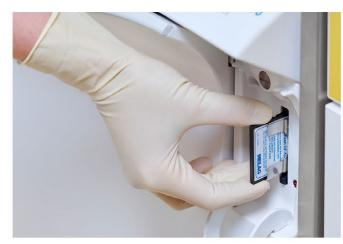
MELAG washer-disinfectors monitor all the relevant process parameters to ensure the highest-possible level of safety. The generated logs **provide legal certainty and can be saved** via CF card or two network interfaces.
