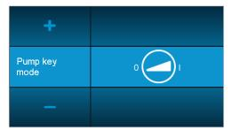
Touch the symbol to change the operating mode of the pump key on the foot control.
