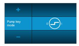
Actuating the pump key gradually increases the coolant flow up to its maximum value.
