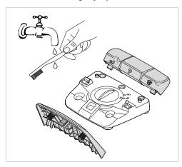
Clean the individual parts of the wireless foot control under running water and then dry them.
