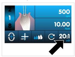
Touch the transmission ratio display to set the value as desired.
