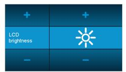
▶ Press the plus and minus keys to change the LCD brightness.
