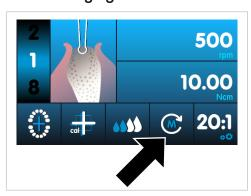
► Touch Direction of motor rotation in order to change the direction of motor rotation.
