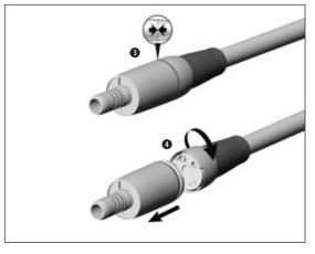
Carry out a visual inspection. The medical device and supply hose coupling must sit flush to one another.
