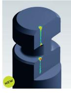
S201L Pro and S201XL Pro: Distribution of the torque over a large surface leads to reduced deformation of the tool edge and, in addition, the load is displaced from the shaft edge towards the centre line. In this manner deformations on the shaft are prevented.
