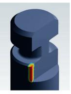
S201 L and S201 XL: A high tool edge load can lead to significant deformation This results in jamming of the clamping system shaft.
