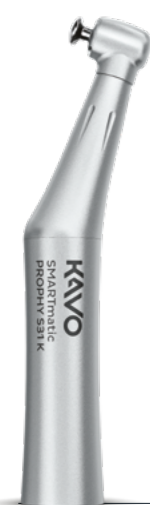
SMARTmatic PROPHY S31 prophylaxis contra-angle (8:1) Double-threaded (1-64-UNC and 1-72-UNF) for screw-type polisher / brushes, unscrewable holder for Snap-on polishing applications, max. drive speed: 20,000 rpm, sealing to prevent intrusion of paste Mat. no. 1.011.6760
