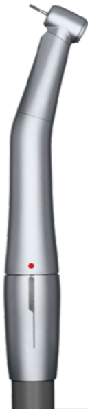
COMFORTdrive contra-angle 200 XD High-speed contra-angle, very light and versatile, integrated brushless motor, glass rod light conductor, ceramic ball bearings, spray filter replaceable by user, 3-port spray, only suitable for direct connection to KaVo COMFORTbase™, max. drive speed: 200,000 rpm Mat. no. 1.000.5500
