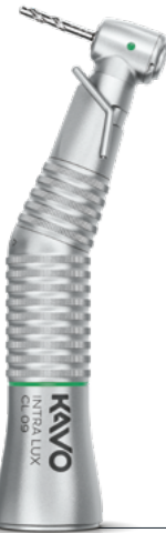
INTRA LUX contra-angle (27:1) Glass rod light conductor, can be dismantled into head and shank, head with internal cooling system (as per Kirschner and Meyer), external coolant connection CL3-09 | Mat. no. 1.002.3693 Consisting of: INTRA LUX surgical reducing head (3:1) CL3 | Mat. no. 1.001.8993 INTRA LUX surgical shank (9:1) CL09 | Mat. no. 1.001.9258
