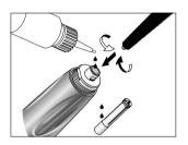
Clean the inside and outside of the shaft using the cleaning brush.
