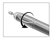
Turn the front sheath anticlockwise until it engages audibly.
