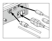
• Connect the motor cable, operating controls (optional), air hose (Perfecta 600) and mains cable.
