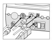
Oconnect the motor cable, operating controls, footoperated starter, air hose (Perfecta 600) and mains cable.
