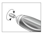
Start the motor handpiece until the required speed is reached. After approx. 2 seconds, an audible signal sounds and the required speed is saved.
