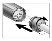
Assemble and tighten the cap.
