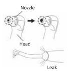
The entire head must be replaced, not only the nozzle.
