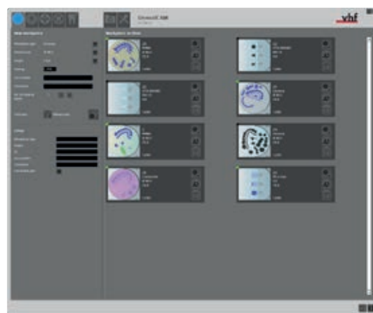
Start screen: easy definition of the characteristics of a new blank at the left side of the window as well as overview of the archive of already existing blanks with various filter functions on the right side.
