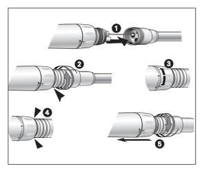
Air motor with fixed connection assembly/removal
