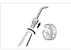
► Slide the nozzle needle into the cannula from the front while rotating it.
