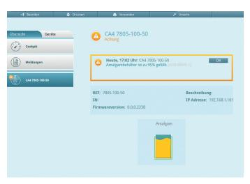
Operating status is able to be monitored via the PC thanks to the Tyscor Pulse.
