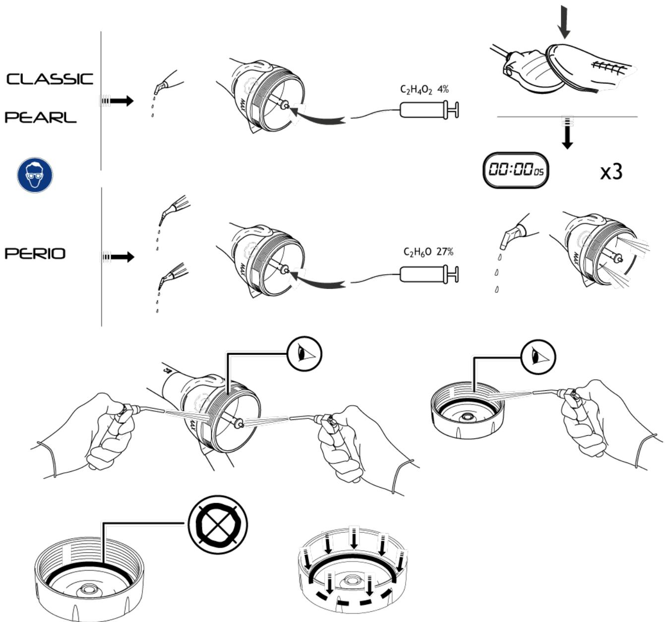
The Classic and Pearl powders are cleaned using a 4% acetic acid aqueous solution.
