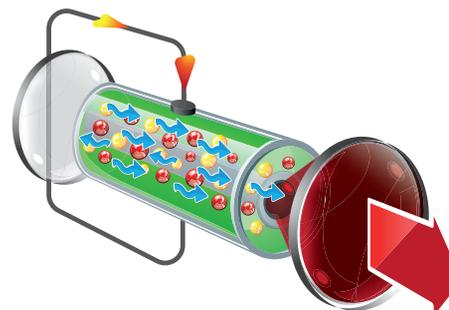
4. The photons exit the optical cavity through the partially reflecting mirror with all the characteristics of a laser
