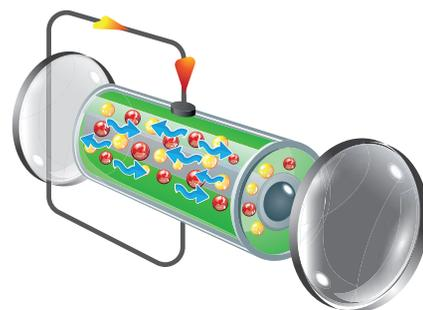
3. The optical cavity mirrors align the movement of the photons
