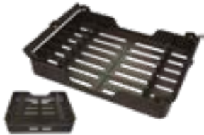
Easy clip tray (empty) 180x136x30mm 8 instruments - Material: PSU 90g
