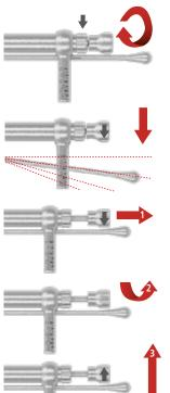
To dismantle the torque wrench for cleaning procedure, unscrew the wheel and then remove the inner bar where the spring is assembled.
